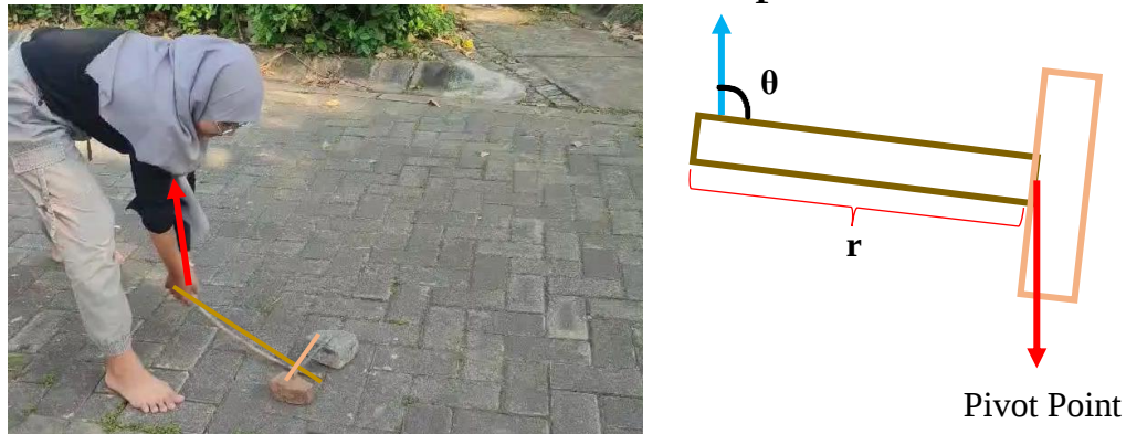
Figure 4. Components of Torque in the Levering Motion of the Short Stick
