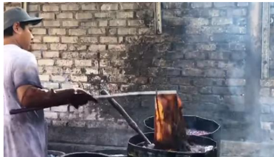
Figure 5. Nglorot Process (Boiling Batik Cloth) (Agnes, 2021)
