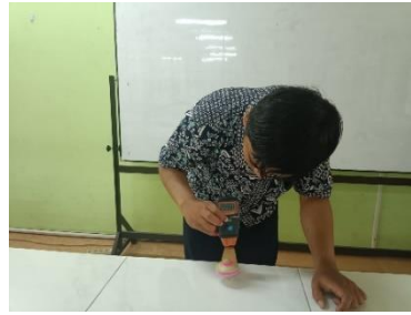
Figure 4. Angular Velocity Observation Using a Tachometer
