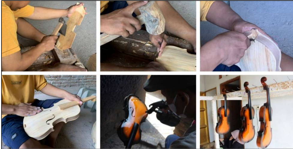
Figure 2. The Process of Making a Violin
